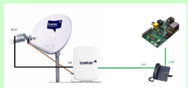
Figure 9: Block diagram of the IP phone system via IPSTAR satellite.
